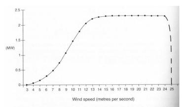
1.4 Typical power curve relating wind speed to electrical output. Data for a Bonus turbine (broken section at and above cut-out speed inserted by author). There is negligible generation below 5 m/s; peak output is not reached until 15 m/s (Beaufort 7 – Near Gale) and at 25 m/s the turbine is shut down for safety.
